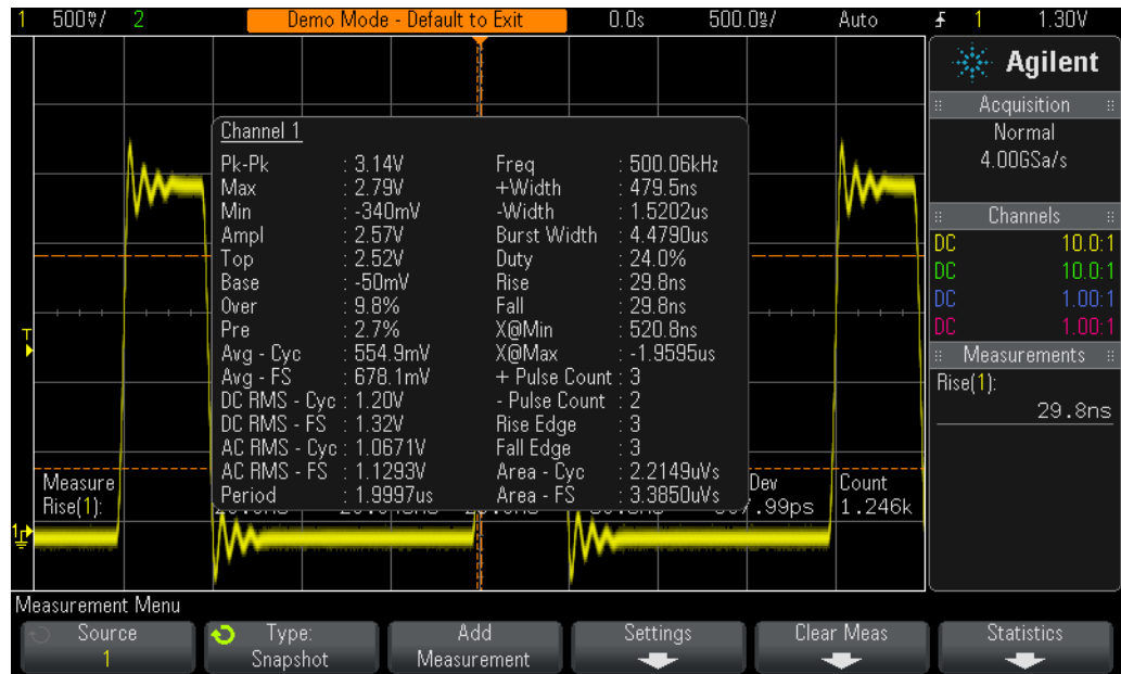
Figure 7 Performing a comprehensive set of automatic parametric measurements using the “Snapshot All” function.
